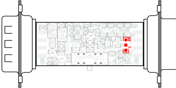
Figure 2: Position of soldering field JP1 on the bottom side of the opened PCAN-AU5790
