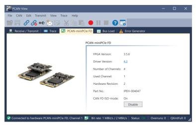
The CAN interface tab shows information about the hardware and the used Windows device driver. In this case exemplary for the PCAN-miniPCIe FD. Depending on the CAN interface, a hardware ID can be determined to distinguish several interfaces of the same type. For interfaces with CAN FD a transmission according to "ISO" or "Non-ISO" can be set as default of the hardware.
