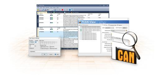
The CAN monitor PCAN-View is a Windows software for viewing, sending, and recording CAN and CAN FD messages. The software is installed with the installation of the device driver package under Windows.
