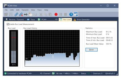
The *Bus Load* tab displays the current bus load, its time history and statistical information of the connected CAN channel.
