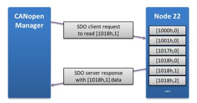
A request could be: "Node number 22, what is your data at [1018h,1]?". If node 22 is present, then it sends a response containing the requested data. Data of 32 bits or less is accessed with a single message pair (request, response). If data is larger, then data gets segmented and multiple request and responses are exchanged.
