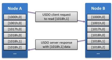
On CANopen FD, this service replaces the SDO. Main changes are that here every node can send USDO requests to every other node and that data sizes in a single request and response scheme can be much bigger, as CAN FD supports large data packages.
