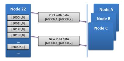
The figure illustrates how node 22 produces a repeated TPDO with the two Object Dictionary entries [6000h,1] and [6000h,2] in it. These can be received and processed by multiple nodes if they have matching RPDO parameters configured.
