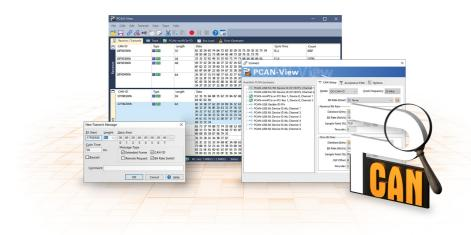
The CAN monitor PCAN-View is a Windows software for viewing, sending, and recording CAN and CAN FD messages. The software is installed with the installation of the device driver package under Windows.
