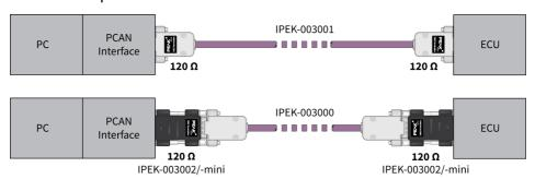
This example shows a connection between the PCAN Interface and a control unit (ECU). The upper example shows a connection with a cable which is terminated with 120  $\Omega$  at both ends. At the lower example the connection is made with termination adapters.
