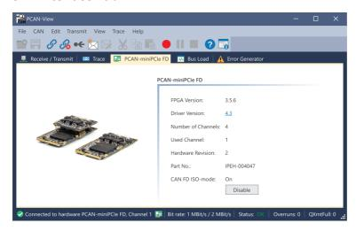
The *CAN interface* tab shows information about the hardware and the used Windows device driver. In this case exemplary for the PCAN-miniPCIe FD. Depending on the CAN interface, a hardware ID can be determined to distinguish several interfaces of the same type.
