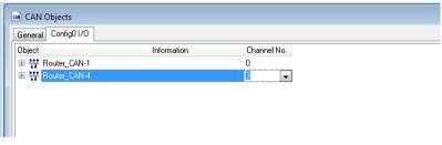
1. Channel-Number: 0 (for Router\_CAN-1) and 3 (for Router\_CAN-4).
